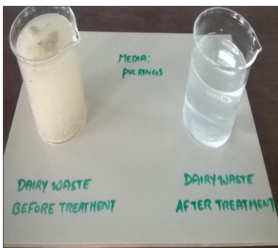
Fig. 3: Sample Before and After Treatment (Using PVC Ring Media).
