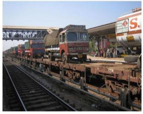
In Konkan Railway system special wagons are used to provide drivable trucks along the entire train on BRN wagon. In this arrangement trucks are loaded through a ramp provided at the dead-end of loop on BRN wagon. These wagons are usually closed coupled to each other with small wheel diameter.
