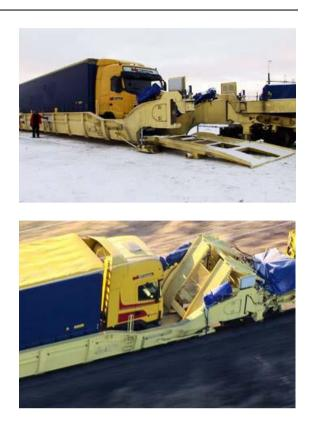
Flexiwaggon combine trucks, buses, cars, containers and Lorries on one and the same wagon. Flexiwaggon mechanism provides great opportunities in transport systems. Flexiwaggon carries the equipments which are necessary for loading and unloading of trucks with the same wagon.
