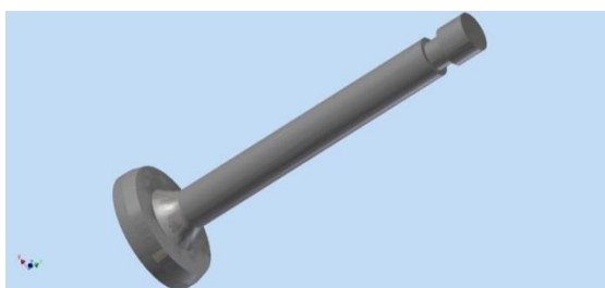
Fig.3: 3D Modelling of Poppet Valve
