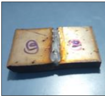
Fig. 1. Weld Bead Geometry Which Includes Width, Reinforcement and Depth of Penetration.
