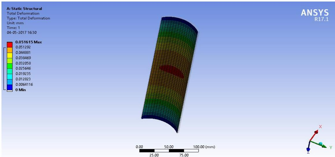
**Fig. 4. Total Deformation of Blade.**
