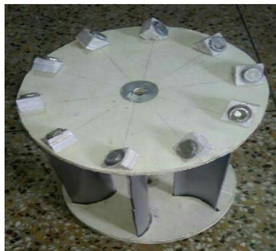
**Fig. 13.** Fabricated turbine.
