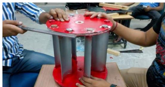
**Fig. 7.** Fabrication of rotor and blade.
