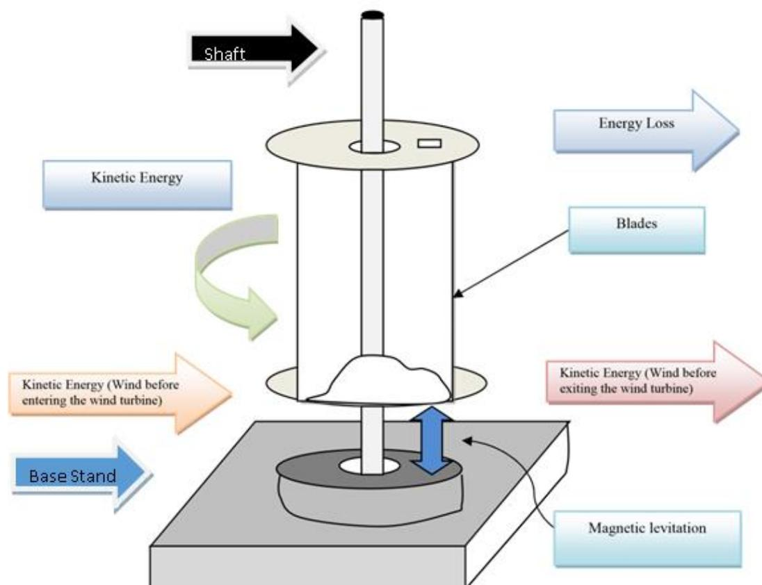
*Fig. 3. Components of a Maglev turbine.*
