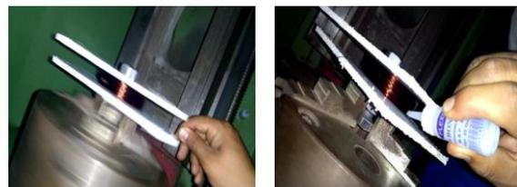
**Fig. 15. Making of coil**
