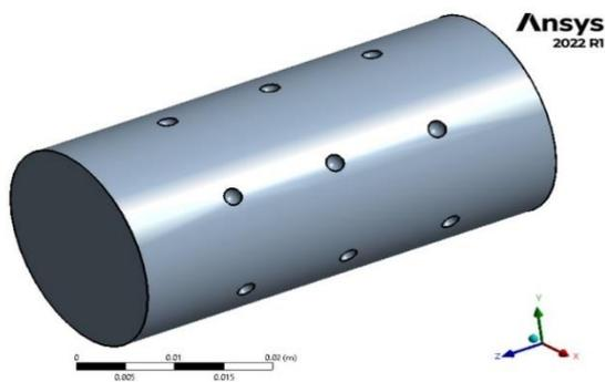
**Figure 4.** Modelling of the fluid domain within the pipe.
