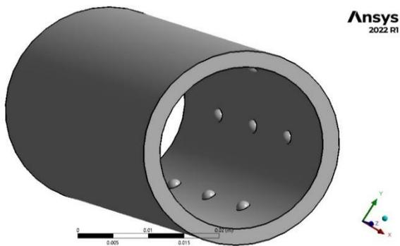
**Figure 2.** Orthogonal views of the dimpled pipe ( $30^\circ$  helical pattern).
