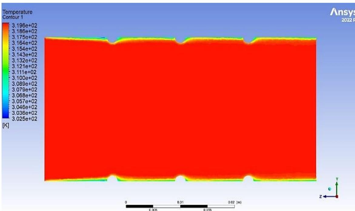
**Figure 7.** Temperature counter of fluid on Dimple pipe.
