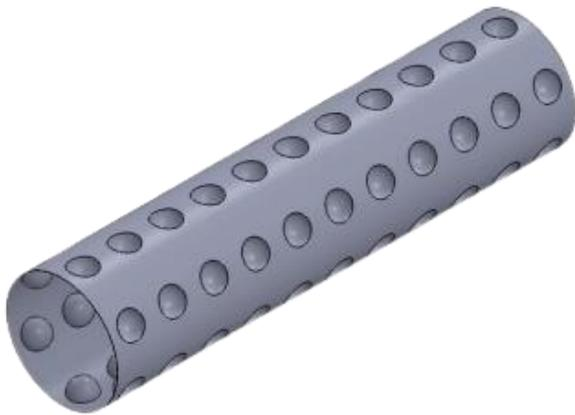
**Figure 1.** Model views of the dimpled pipe.
