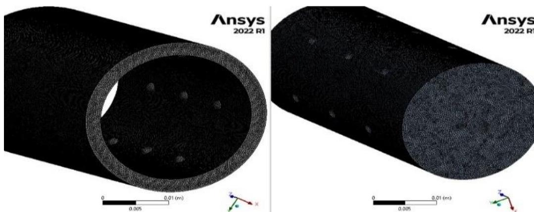
**Figure 5.** Meshed Model of the dimple pipe and fluid domain.
