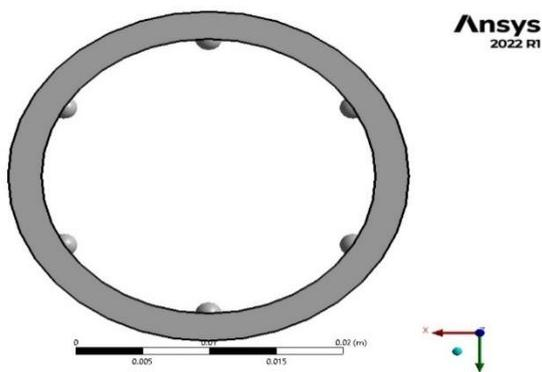
**Figure 3.** Front views of the dimpled pipe. ( $30^\circ$  helical pattern).
