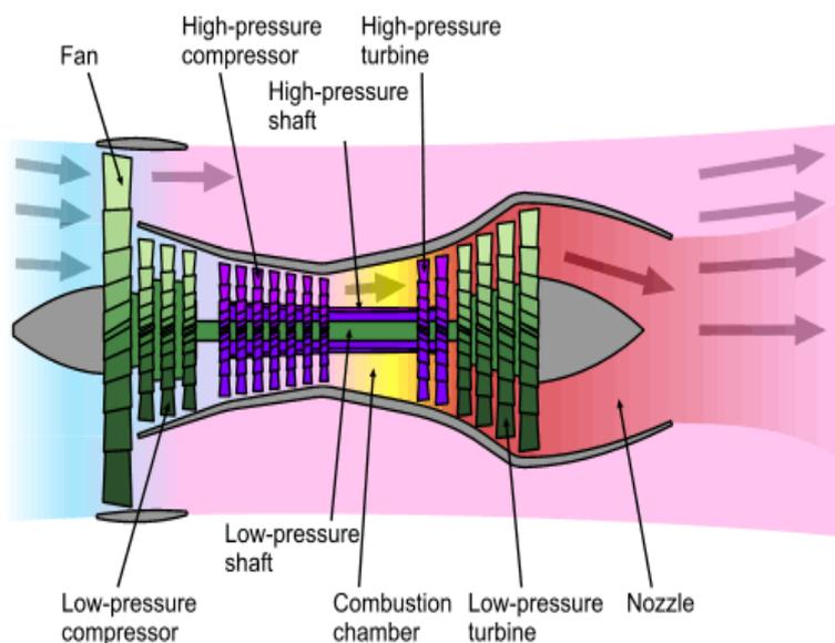
**Fig. 1.** The general view of a turbofan engine [18].
