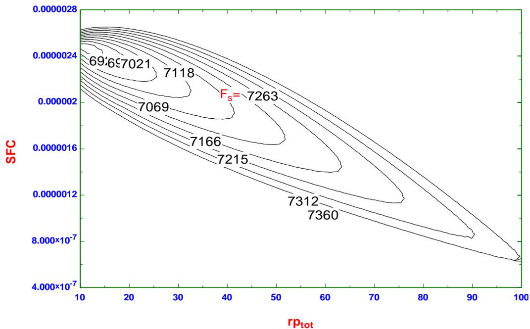
**Fig. 6.** The relationship between the ratio of the total pressure, thrust and specific fuel consumption in general state.
