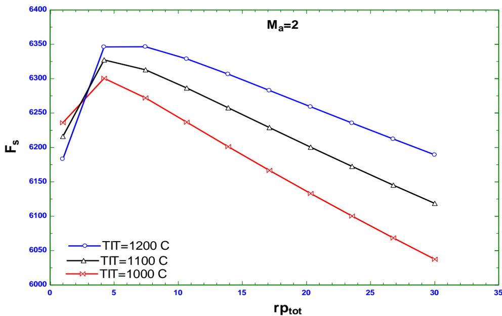
Fig. 4. Thrust changes in terms of the total pressure ratio at a constant Mach.
