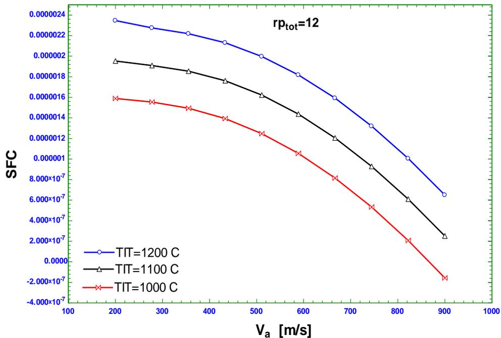
Fig. 3. Specific fuel consumption changes in terms of flight speed at a constant total pressure ratio.
