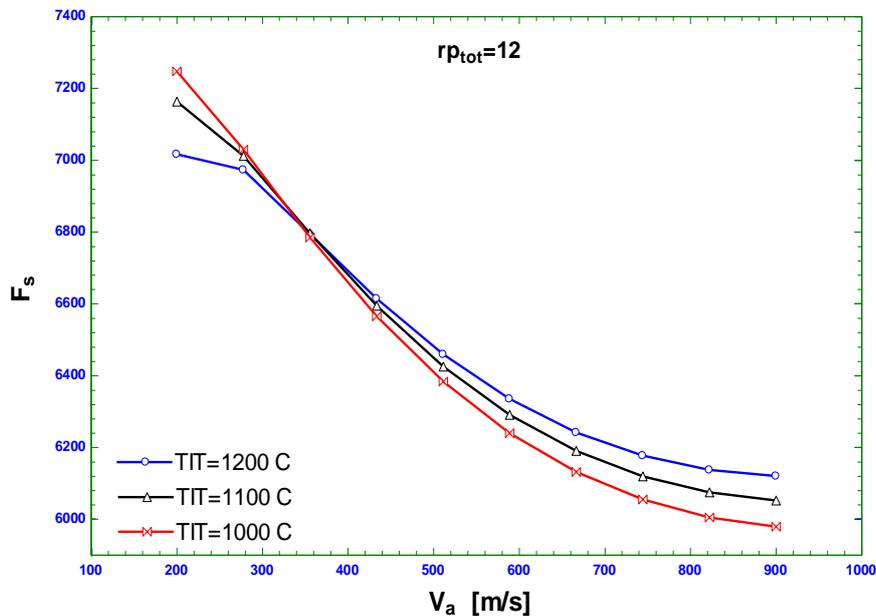
Fig. 2. Thrust changes in terms of flight speed at a constant total pressure ratio.
