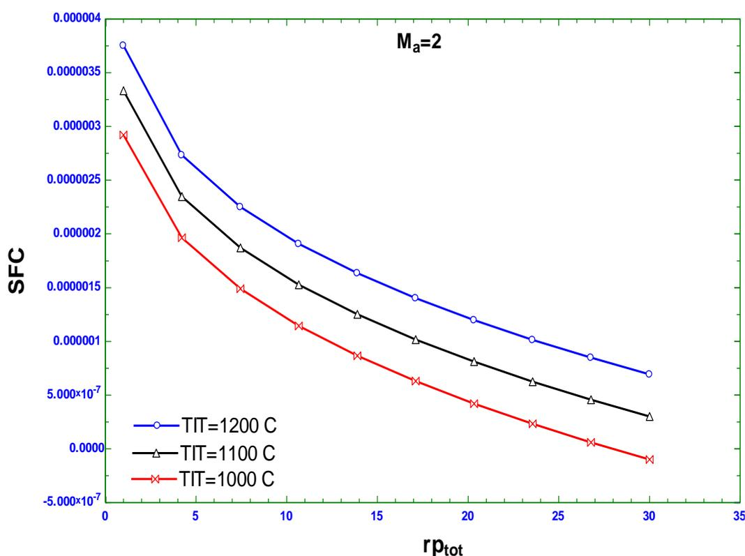
**Fig. 5.** Specific fuel consumption changes in terms of the total pressure ratio at a constant Mach.
