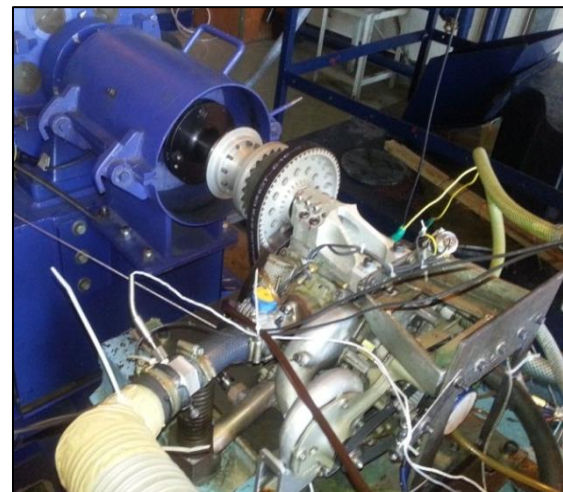
Fig.2: Prototype Wankel engine on Test Bed.
