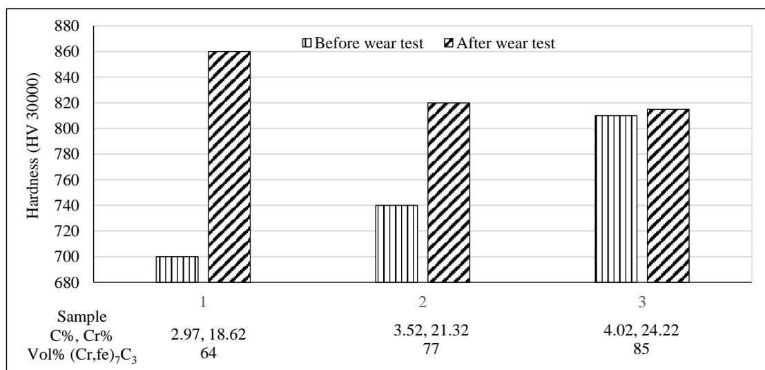
**Fig. 3.** Hardness values for hypoeutectic, eutectic, and hypereutectic samples of Fe–Cr–C. The lower carbon content alloys showed significantly higher hardness values after the wear testing [3].
