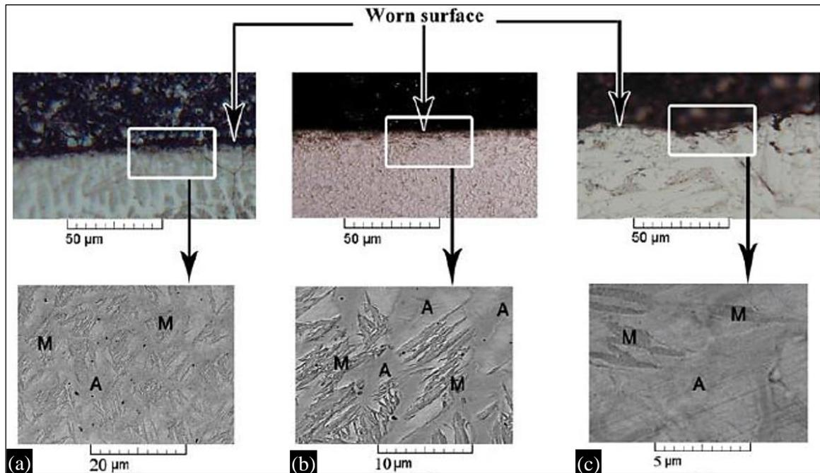
**Fig. 4.** Optical microscope and SEM images of worn (a) hypoeutectic, (b) eutectic, and (c) hypereutectic samples. The M refers to martensite structures and A refers to austenite regions.
