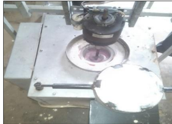
Fig. 1. Melting of 6061 Aluminium Alloy and Stir Casting Setup.
