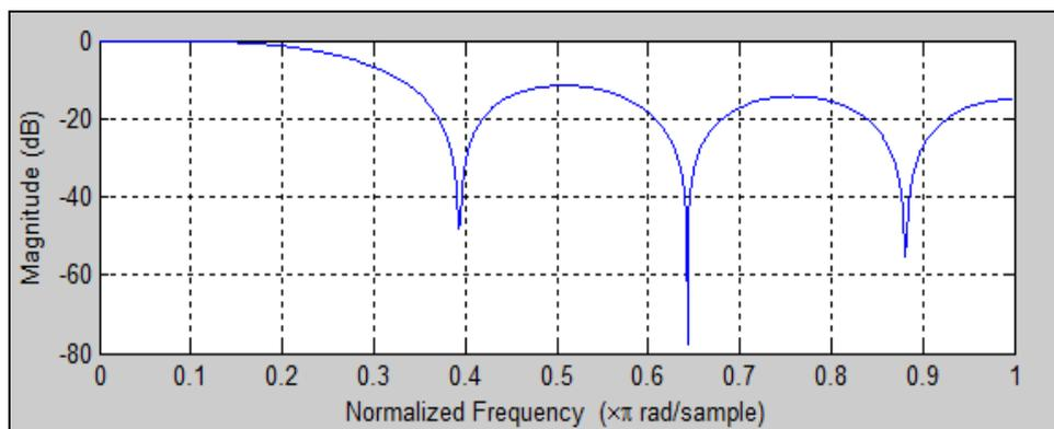
Fig. 2: Frequency Response of the Savitzky-Golay Filter.
