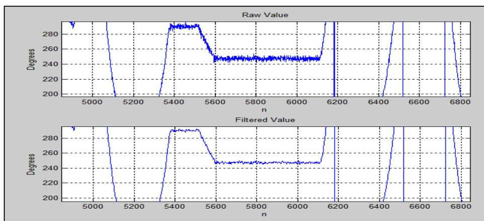
Fig. 6: Savitzky-Golay Filtering Results.
