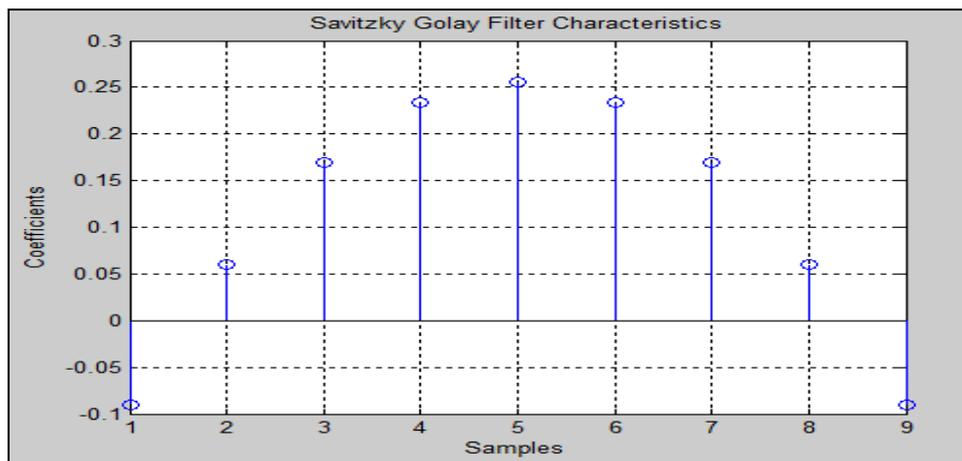
**Fig.1: Savitzky-Golay Filter Characteristics–Time Domain.**
