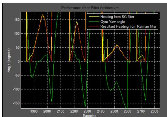
**Fig. 7:** Performance of the Savitzky-Golay-Kalman Filter Architecture.
