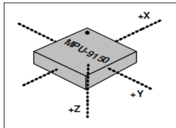
Fig. 4: MPU 9150 Magnetometer Axes Configuration.
