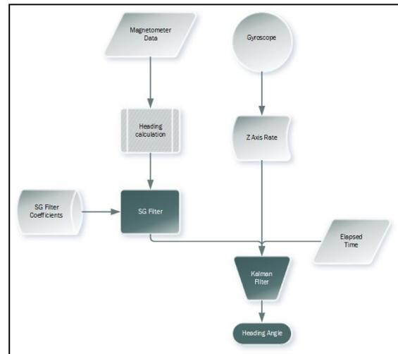
Fig. 3: Flowchart of the Filter Architecture.
