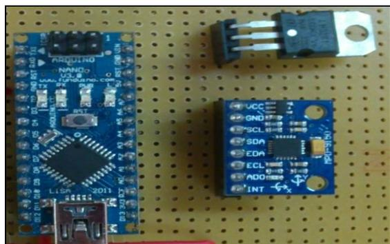
Fig. 5: Evaluation Board with MPU 9150 Interfaced Arduino Nano.
