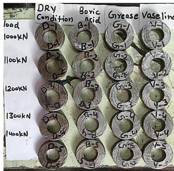
Fig. 4. Specimens after compression.
