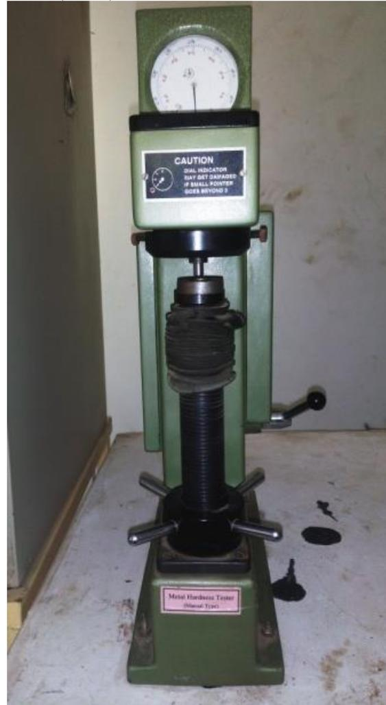
*Fig. 3. Rockwell hardness test.*
