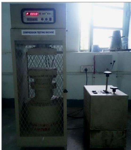
*Fig. 2. Compression testing machine.*
