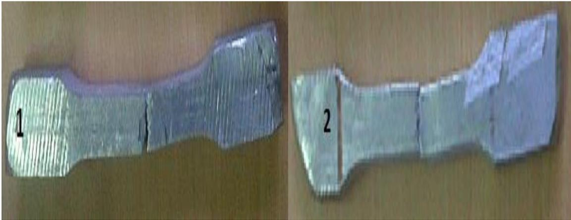
**Fig. 3.** Specimens after breakage.
