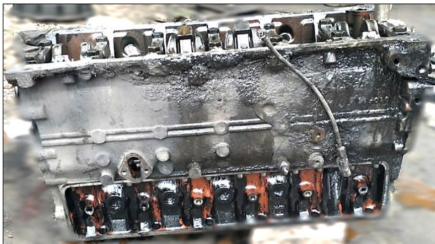
Fig. 1. Engine block during dismantling.
